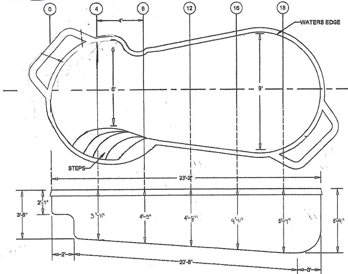
It is important to have your excavator call to review the Dig Diagram prior to excavation. All dimensions are Approximate. A 3" over dig must be added to the bottom for the stone, along with a 2' by 3' trench from the pool hole to the area of the equipment placement for plumbing and wiring.
