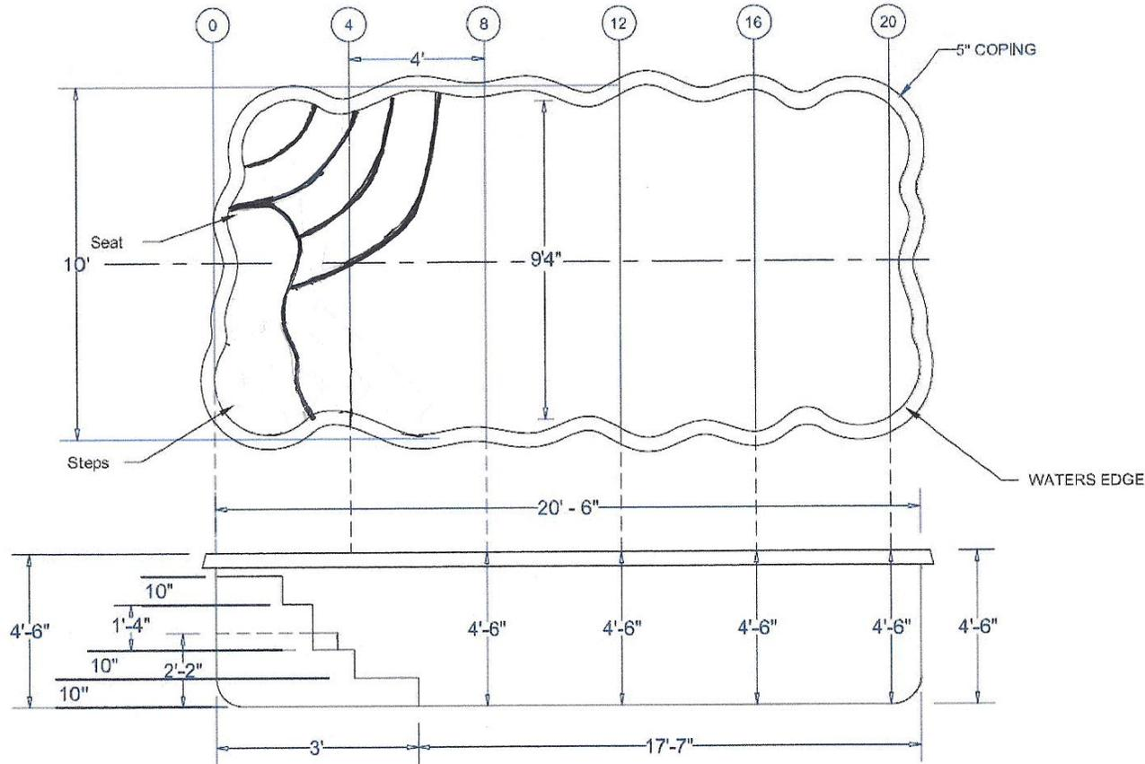
It is important to have your excavator call to review the Dig Diagram prior to excavation. All dimensions are Approximate. A 3" over dig must be added to the bottom for the stone, along with a 2' by 3' trench from the pool hole to the area of the equipment placement for plumbing and wiring.
